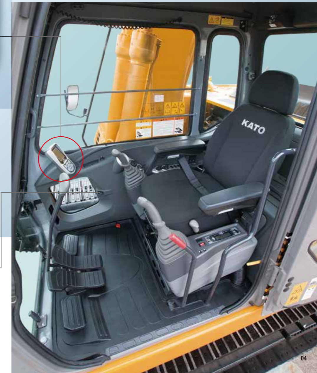
▲ Hour meter The location of hour meter is improved so as to confirm conveniently from outside of the cab.
