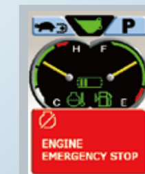
◀ When engine emergency stop switch is operated
