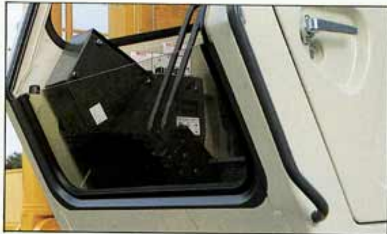
• Crossbar eliminated for wide forward visibility
