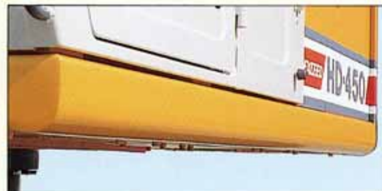
• Sturdy frame-structure prevents the engine cover from the damage
