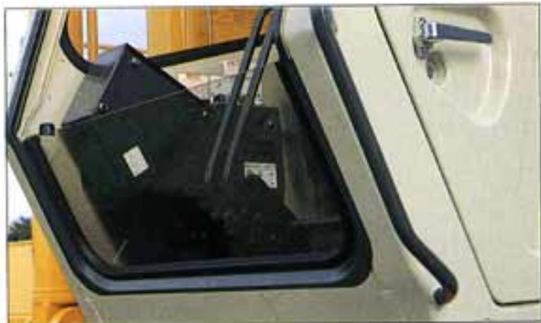
• Crossbar eliminated for wide forward visibility
